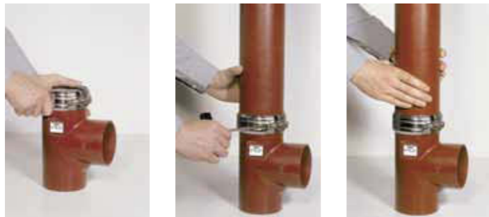
Push the supplied assembled coupling onto the pipe spigot so that it abuts on the central register of the elastomer gasket.
